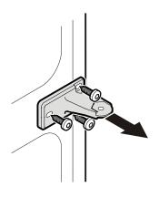
**11.** Pull out the spring mechanism from the refrigerator door and transfer to the opposite side.
