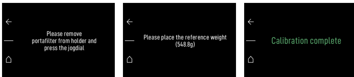
Figure 17; Load Cell calibration process
