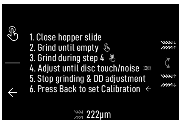
Figure 18; Disc Distance Calibration Process
