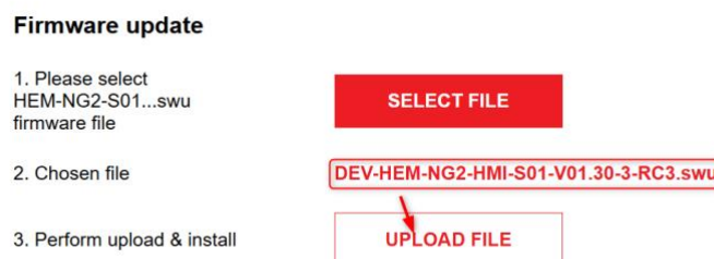
Figure 33; Upload .swu file to the grinder
