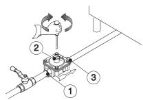
**NB!** These models are designed and certified for use with natural or propane gas. For natural gas, the pressure regulator on the header is set to 8" w.c. (0.1 mbar).
